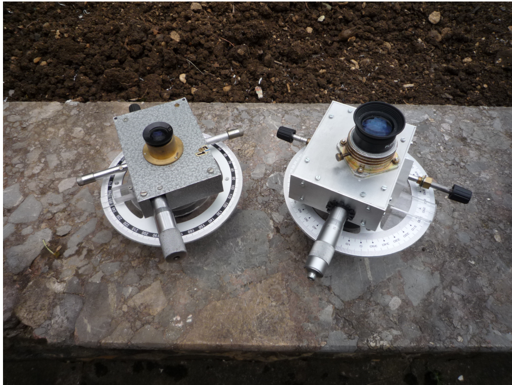
Figure 1: Homemade filar micrometers for the 11-inch telescope
