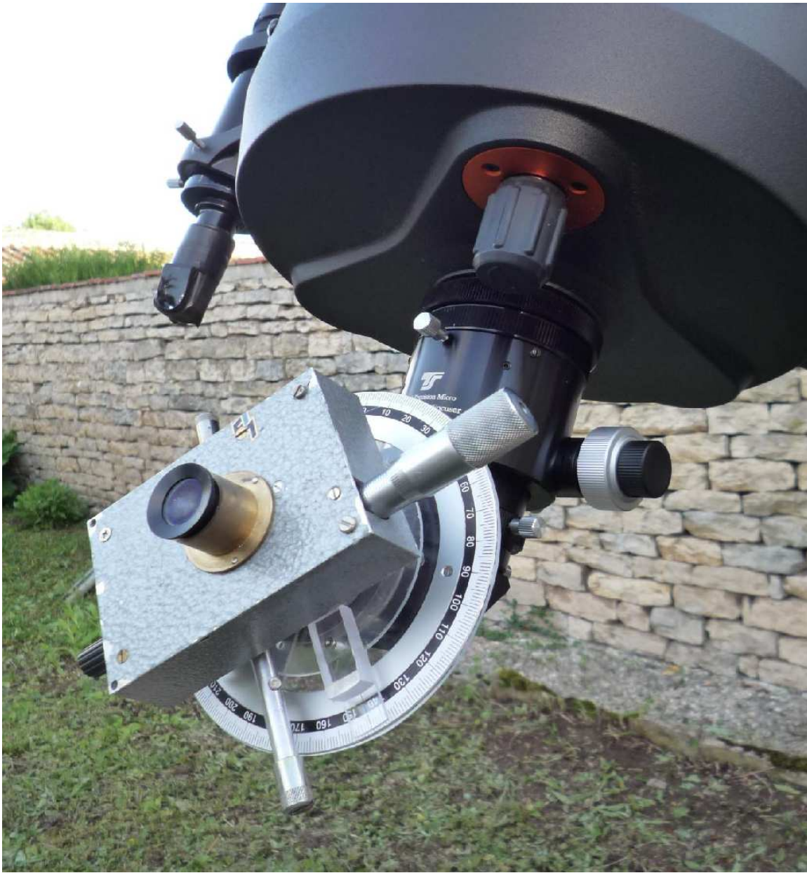
Figure 1: Home-made filar micrometer attached to a 279-mm (11-inch) Schmidt-Cassegrain Telescope (S/Fh in table 1).
